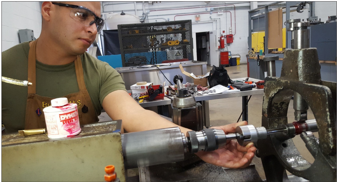
GySgt Ramirez conducting lathe work chambering a barrel for the Marine Corps Rifle Team.
