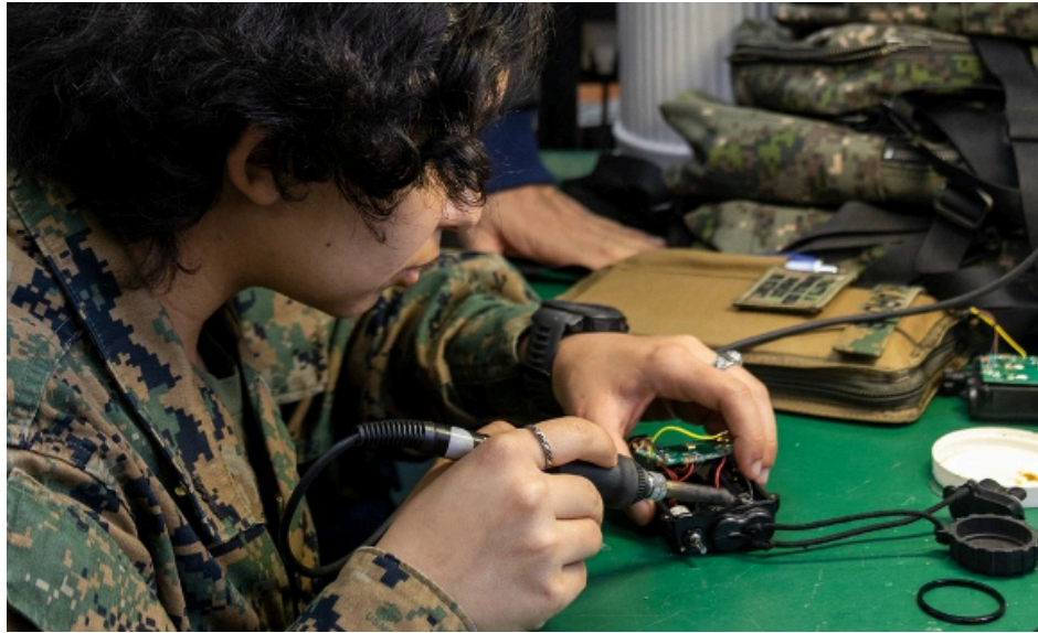
Corporal Eskarous, an electro-optical ordnance repairer, conducts wire repair on ROK-MC NVGs
